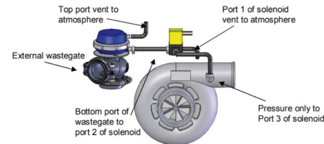
If you are unable to achieve your desired boost pressure, i.e. boost level is too low, or not controllable, it is normally due to exhaust manifold backpressure forcing the internal wastegate to open. To increase your boost pressure further, it is recommended that the wastegate/actuator spring be changed to a spring which is closer to the desired boost pressure. Alternately trial a two-port connection method.
