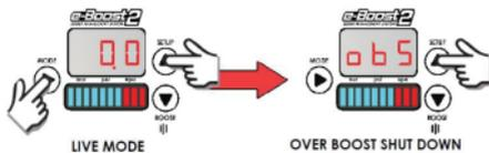
Safety First: This is the limit you will need to set at which your e-Boost2 will cut boost for safety reasons. **THIS MUST BE SET UP FIRST OR YOUR ENGINE WILL NOT PRODUCE ANY BOOST.**
