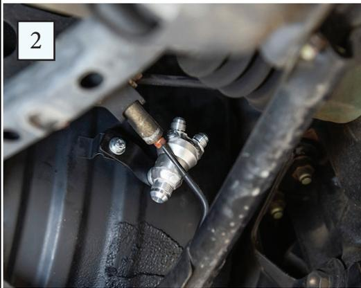
If you have purchased the complete fuel system package you will now install the supplied 3-way distribution block which bolts it in place to the factory mounting point found beside the rear brake line splitter with the supplied mount (See pic 2.0).
