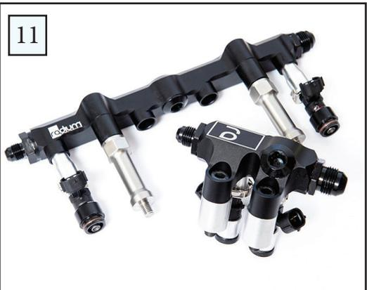
To make the job as easy as possible, the injectors and rails are supplied assembled with the correct spacers, block-offs & fittings in place so the whole assembly is ready to just drop in place of the factory setup.
