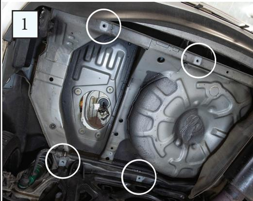
Being an under-car tank, the fuel lines will need to be installed first, before the tank is raised up into place. If you have purchased the fuel tank combo by itself and are sorting your own fuel lines, you will need to dummy the tank up in place to begin with to measure your lines.
