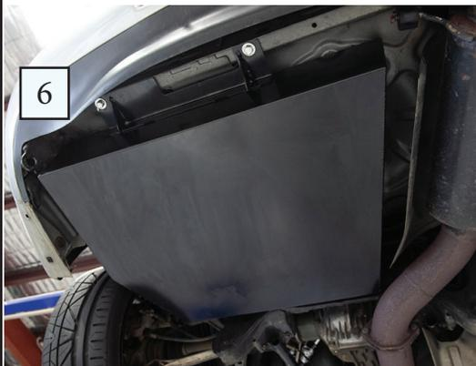
With the fuel lines, sensor & fuel filter all mounted in place, the tank can now be raised into position and bolted into place. Supplied pre-assembled and ready to go, the FD3S RX7 Fuel Tank set-up is a bolt-in replacement for the OEM tank, utilising the 4 factory M8 mounting points (see pic 1.0)
