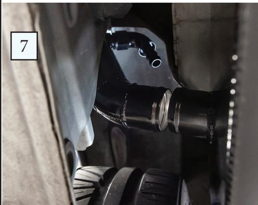
The fuel filler neck can now be installed from the underside of the rear quarter using the stainless allen heat bolts supplied. Due to space restrictions (see pic 7.0) the joiner hose needs to be slid onto the end of the fuel tank inlet prior to installing. Once the filler neck is in place, the hose is then slid over the filler neck & clamped in place. A light smear of lubricant over the filler neck tube & tank inlet will allow the hose to be positioned easily.
