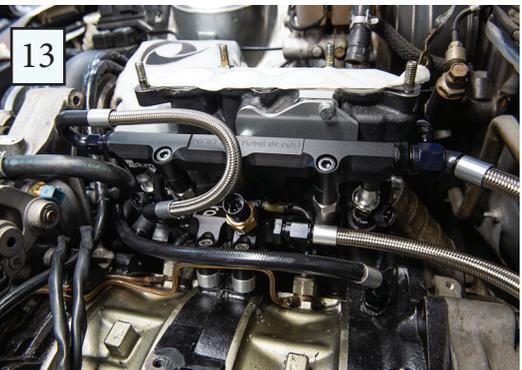
With the injectors and fuel rails now in place, the plumbing can now be finished up. All fuel lines are supplied labeled, ready to screw in place onto the primary & secondary fuel rails.
